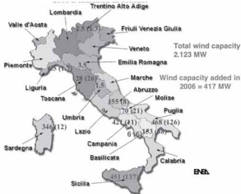
Figure 6 Wind capacity at regional level in Italy at the end of 2006 in MW. Wind capacity added in 2006 is indicated in bracket.
