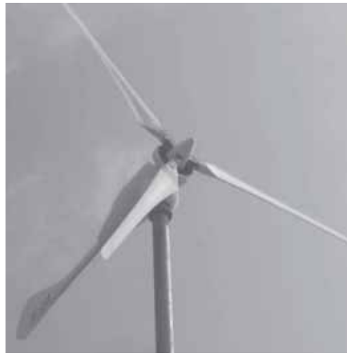
Figure 9 BMP 20, the 20-kW prototype developed by BluMiniPower srl.
