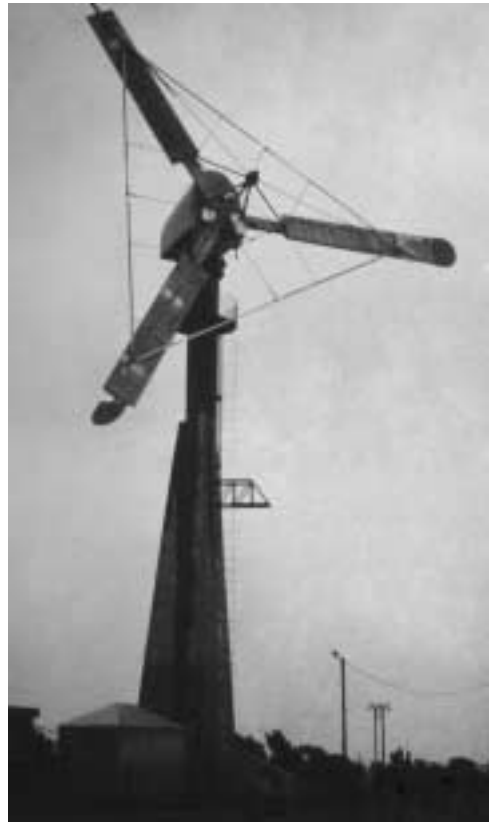
Figure 3.3 The refurbished 200-kW Gedser machine operated for 650 hours between November 1977 and April 1979, when it was taken out of service. Total power production was 39,890 kWh.
