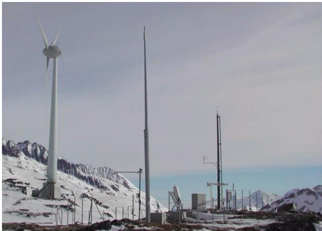
Figure 2. Installation on Mt. Gütsch with Enercon E-40 and test bench of the Swiss Met Institute and results of collecting samples of ice throw
